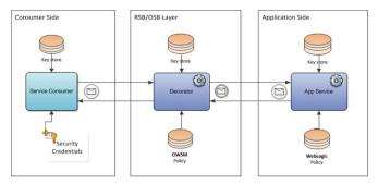
The RSB key components can be loosely coupled across platform, technology, and physical topologies. In order to establish an end-to-end security in RSB system, one has to secure all the intermediary layers that are part of a communication channel through RSB. As discussed earlier, there are three main layers, Service Provider, Decorator and the Service Consumer. Each of these must participate in configuring security in order to achieve effective security while making Web service calls.
